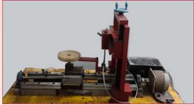
Low Speed Reciprocating Piston Test Rig
