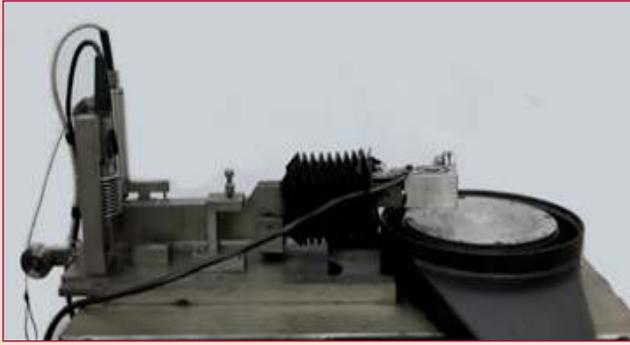
Pin on Disc Tribometer
