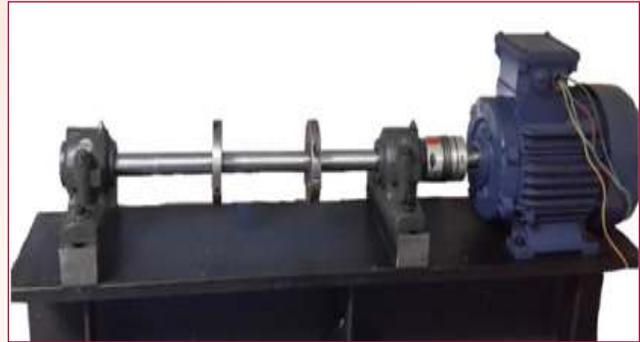
Bearing Fault Detector Test Rig
