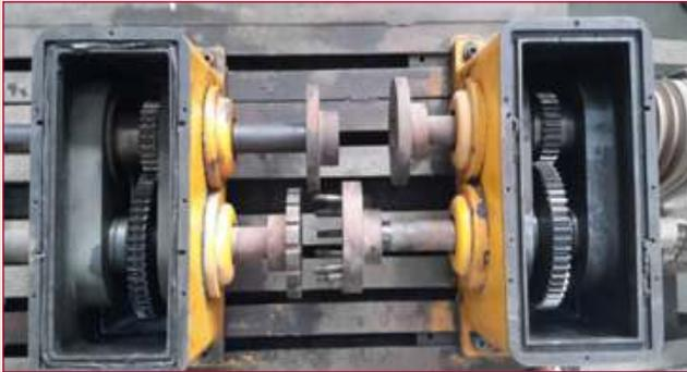
FZG Gear Test Rig
