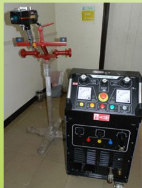
Wire Spray Facility
