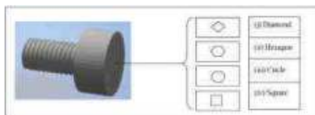
Fig. 3 - Different Patters engraved in a array on the screw face
