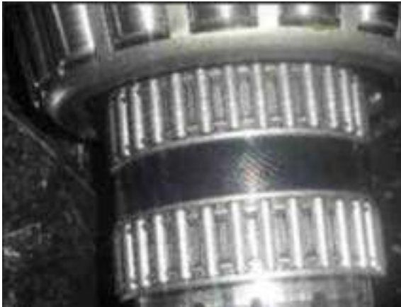
Figure:7 - Post Test picture of NRBs made as per recommended specifications.
