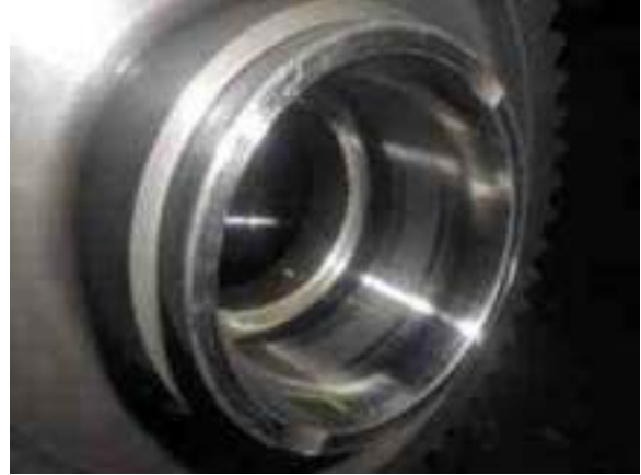
Figure:8 - Tested gear bore with new Needle Roller Bearings
