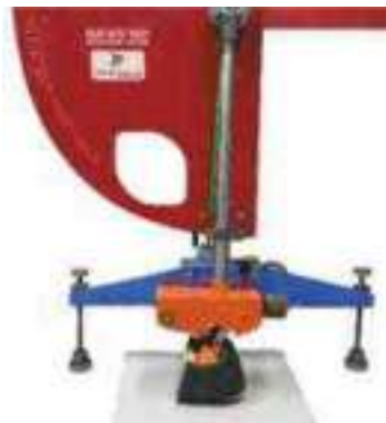
Figure 1: British Pendulum skid tester with modified shoe outsole arrangement
