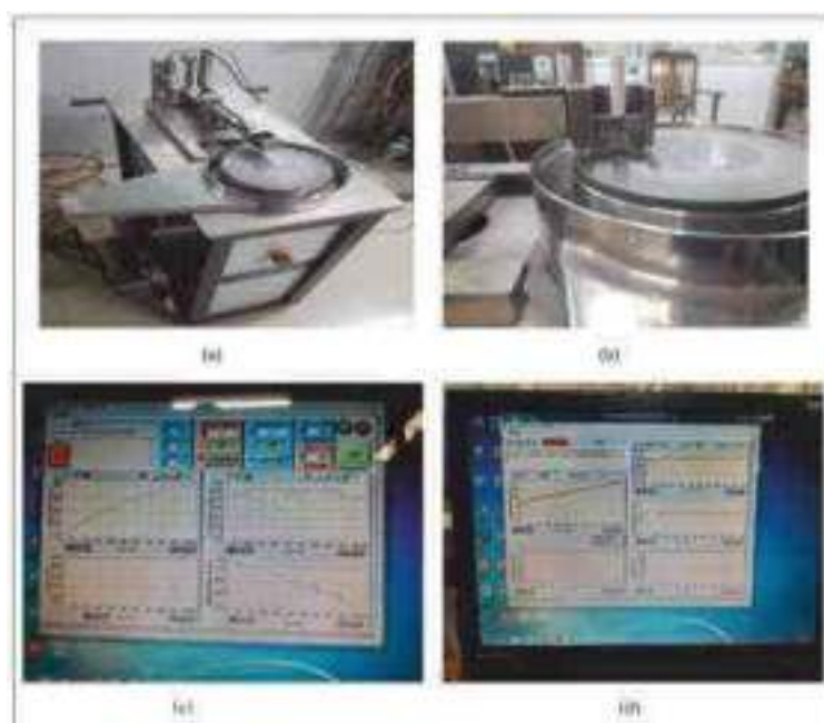
Fig. 6 – (a) Pin on disk friction and wear monitor(Manufacturer- DUCOM,2013); (b) PLA Sample inserted in the holder ; (c) Pin on disk friction and wear monitor control interface ; (d) Outputs obtained on monitor.
