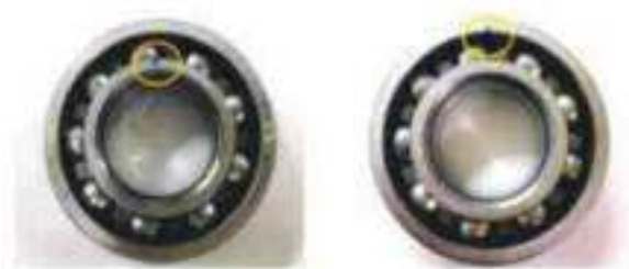
Figure 2: Defects in (a) Inner race (b) Outer race in SKF ball bearing
