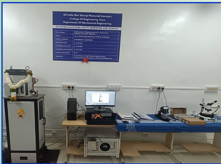
Four ball tester, KRL shear stability tester, Image acquisition system, Digital Microscope
