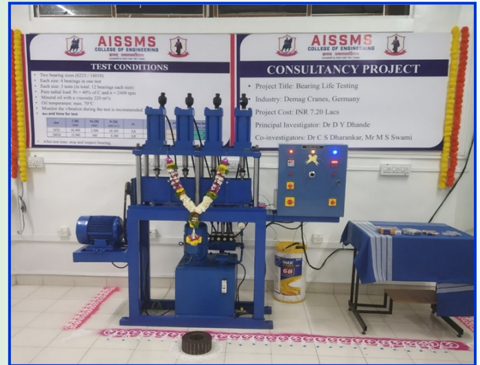
Bearing test rig developed as a part of an overseas consulting project from Demag Cranes, Germany.
